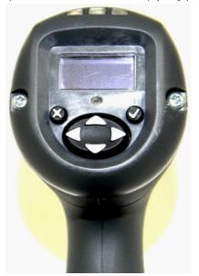
2. Using a T-10 Torx Bit remove the two display panel screws.
