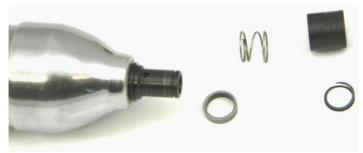
1. For units with the \%"quick change spindle, disassemble the spindle as follows. Remove the spiral spring clip from the front of the spindle, then remove the quick change collar, spring, spring support and rear spiral snap ring.
