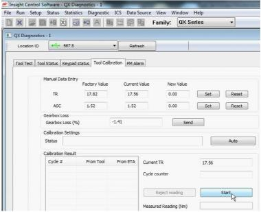
6. Click on the start button to begin the test and then run 10 runs at 100% torque on a medium test joint, then click on the stop button.
