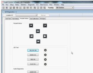
8. Under the Keypad Status tab check the functionality of each of the keypad buttons and lights by clicking on their corresponding buttons on the screen. Now close ICS and disconnect the Tool.
