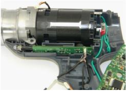
8. Connect the second connection from the end of the Interface Cable to the trigger board, and insert the trigger board into the housing.
