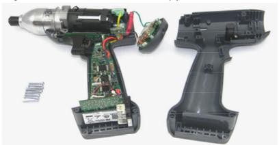
19. Install the second half of the housing onto the unit by tilting the bottom of the housing and align the housing and the foot PCB. Slightly push forward on the board to ensure it seats into the slots in the housing.
