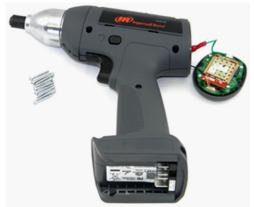
21. Install the housing screws in the tool to 1 Nm. Starting with the center screw, then the top two screws, proceeding to the middle and finishing with the bottom to screws.
