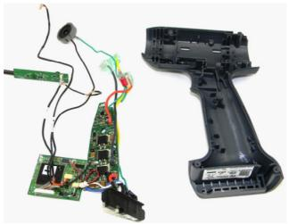
13. Carefully remove the electronic components (circuit boards, transducer and cables) from the housing.
