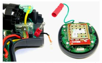
5. Disconnect the pin connector first, then disconnect the ground wire slip connector. Remove the USB port cover from its slot in the housing.
