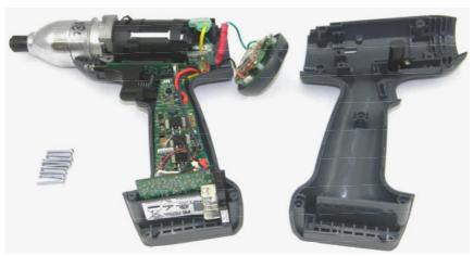
4. Carefully remove the housing clamshell ensuring that you do not damage any of the cables or connectors.
