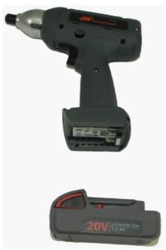
1. Remove the battery from the tool, and place the tool on the work bench with the Display facing up.
