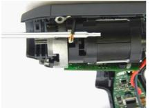
7. Remove the hall cable connector from the motor. This connector is located at the top of the motor. It should be removed by placing the shaft of a small screwdriver under the cable to support it just behind the connector then gently pulling up on the screwdriver to unplug the connector.
