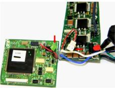
17. Disconnect the Handle PCB from the Foot PCB at its connector. This completes the disassembly of the electronic components.
