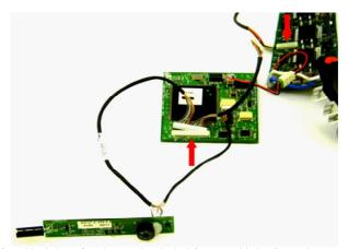
15. Disconnect the Interface cable which runs from the trigger board to both foot PCB and the handle PCB. There is one connector on the foot PCB and one on the handle PCB.
