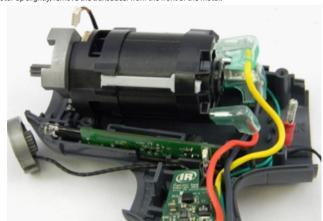
11. Unplug the three motor terminals from the rear of the motor, by pressing the locking detents on the connectors under the clear boots. Note the orientation of the three terminals. They must be installed in the same orientation when the tool is reassembled. Now remove the motor from the housing.
