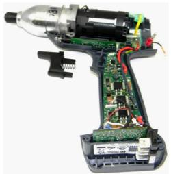
6. Remove the trigger by pulling the trigger up slightly and out of the housing. Also remove the reverse lever from the housing.
