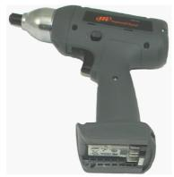
3. Using the same screwdriver now remove the housing screws. Remove the bottom screws first, followed by the top, middle, and finally the center screw.
