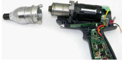
8. Tilt the motor and gear case assembly up at a slight angle, then carefully remove the gear case assembly from the motor.
