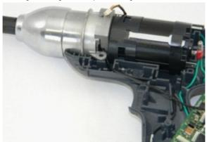
7. Install the motor/gear case assembly into the Housing. Seat the rear of the motor first then, carefully lower the assembly into position. Add a service loop to the transducer cable under the gear case ear. Ensure that all the cables are clear of the assembly and that they have not been pinched or cut. Also be sure that the assembly is fully seated in the housing.
