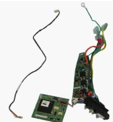
16. This will leave the Hall Cable which can now be disconnected from the foot board and the cable removed.
