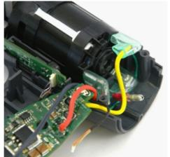
13. Connect the three motor leads, in their proper orientation. The black lead is connected to the bottom lug (closest to the housing). The yellow lead to the top lug, and the red lead to the middle lug (closest to the trigger board). There are also markings on the housing halves to aid in the orientation of these leads. Also ensure that the terminals are connected at the proper angle.
