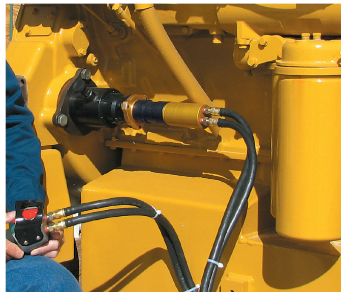
A B006PVR374-03-31P barring motor using pendant control, slow turning a Caterpillar 3408 engine.
