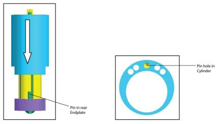
5. Place Front Endplate (with Wave Washer and Bearing) assembly onto rotor shaft. Align roll pin (8b) in cylinder assembly with pin hole in front endplate.
