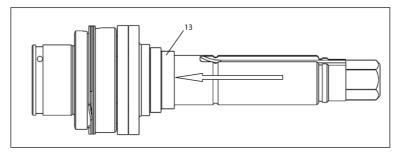
13. Slip Collar Spring (2) over Drive Shaft. Flat face of Collar Spring Must Sit on the Step of Shutoff Collar.
