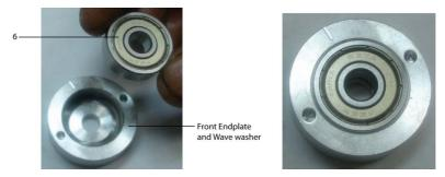
4. Place above assembly in the counter bore of fixture 80187420. Kidney slot side of front endplate must be upward.
