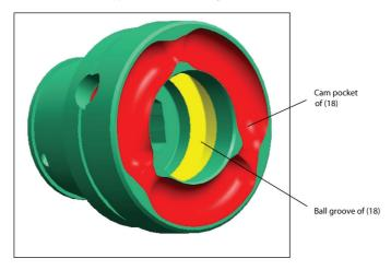
2. Fill Ball Groove and Plunger Hole of Driver Shaft (9) with Ingersoll Rand # 40036-1 Grease.
