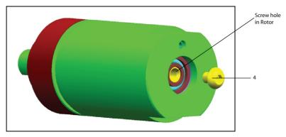
5. Slowly tighten Adjustment Screw. Tighten it until Assembly rotates freely.
