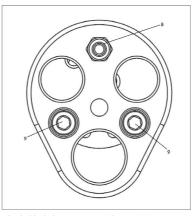
8. Insert Chip Holder Assembly (2) into the chip holder hole in remote start housing (1).
