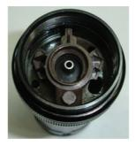
7. Coat Reverse Screw (8) Threads with loctite # 542. Tighten reverse screw fully with allen key on reverse ring assembly placed on motor housing and then back off 1 / 4 turn. Make sure that screw sits over reverse valve edge. Remove the excess loctite.
