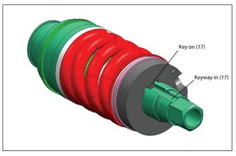
21. Grease Ball Race of Adjustment Nut (5) with Ingersoll Rand # 40036-1 Grease and place 22 X Ball 2.78mm (20) in it.
