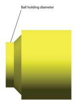
2. Hold Ball Seat (2) on Ball Seat Assembly tool (OM127) as shown in picture below.
