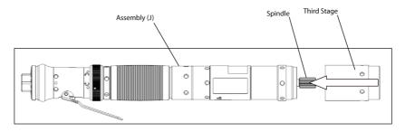
2. Mount Spacer (QA8-208) in Gear case (QA8-31-37) of the Third stage assembly (QA8-M37-4P29-1) for QAAA..150.. and QAAS..090.. models.
