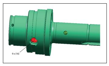
once all balls are removed, separate Driver Shaft (9) from Upper Driven Jaw (18).
