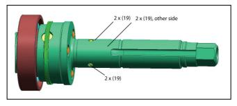
9. Remove Retaining Ring (Qa8-701) from upper driven jaw's (18) retaining ring groove.
