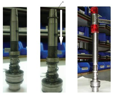
Note: 1. Check That Retaining Ring (4) is Correctly Positioned onto Driver Shaft's (9) Groove. 2. Make Sure that the Plunger Positioned in Steps 10 and 11 is in its Position.
