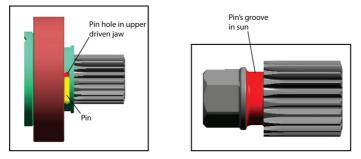
3. Place Retaining Ring (QA8-701) onto retaining ring groove of Upper driven jaw to Pin (QA6-15) in place.
