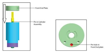
6. Place Fixture 80187420 on top of motor, then press until bearing (6) is properly spaced.
