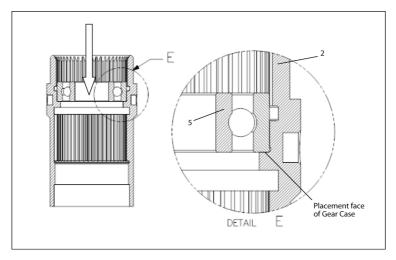
2. Grease Gear Case's (2) Splines with Ingersoll Rand # 90 Grease. Place Spindle Assembly (3) onto bearing in gear case with hand first and then press using manual press to butt against the placement face of bearing. Support bearing inner race during pressing. See section and detail views below for the placement.
