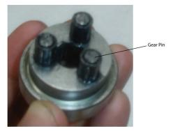
2. Place Planet Gear, Qty # 3 onto Needle Roller Bearings of above Assembly.
