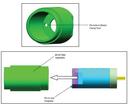
Thread Back Cap onto fixture. Tighten it to 40 nm (30 ft-lb) using a wrench. Note: Motor clamp tool fixture simulates motor in actual tool assembly. Unclamped motors may not be properly spaced and cause motor to overheat or bind.
