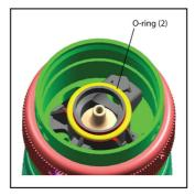
2. Mount Valve Seat (1) over The O-ring of above Assembly. Make sure that the O-ring (2) sits on the o-ring diameter of valve seat.
