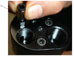
2. Tighten Tube Fitting (3) onto Primary exhaust hole threads in Remote Backend Housing clockwise using Adjustable spanner wrench.
