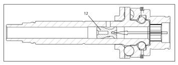
11. Grease 3 X cross holes of driver shaft with Ingersoll Rand 40036-1 Grease and Insert 2 X Plunger Ball 2.38mm (19) Per Hole. See section view below for the proper placement.
