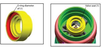
3. Place Shut-off Valve (4) on the shut-off valve groove of valve seat (1) of above assembly. Make sure that stem of shut-off valve passes through the hole in valve guide in motor housing.
