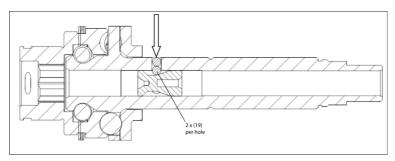
12. Grease I.D of shutoff collar (13) with Ingersoll Rand # 40036-1 Grease. Slip shutoff collar over drive shaft.
