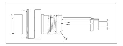
15. Use Retaining Ring tool (80187362) to place Retaining Ring (4) on Driver Shaft (9) Groove.
