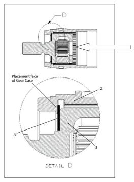
4. Grease Spindle Assembly's (3) gears with Ingersoll Rand # 90 grease.
