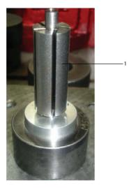
6. Oil all surfaces of new vanes (Qty # 5) with Ingersoll Rand # 10 oil. Place them one at a time in rotor (1). Make sure to match vane profile radius with profile radius of rotor.
