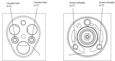
7. Tight screw (8) clockwise to 5 nm (3.7 Ft-lb) and screws (9) clockwise to 6 nm (4.5 Ft-lb) assembled in step 5 and 6 by using a torque wrench.
