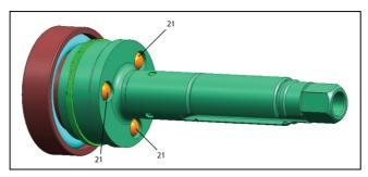
Remove 6 X Ball 2.78mm (19) from clutch shaft's plunger holes. Note: Check that there are 6 balls and keep them for re-assembly unless heavily worn.
