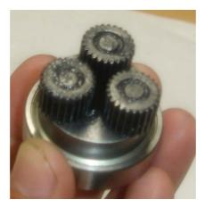
3. Grease Gear Case's splines with ingersoll rand # 90 grease. Place above assembly in gear case (5).Ensure planet gear's teeth engage with gear case's teeth and face of bearing in spindle assembly must sits against the placement face of gear case. See section view below for the proper placement.
