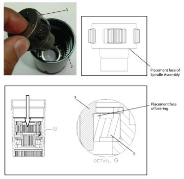
4. Grease Spindle Assembly's (3) Gears with Ingersoll Rand # 90 Grease.
