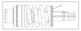
20. Slide Lock Nut Washer (17) onto above Assembly. Align Key on Lock Nut Washer with Keyway In Driver Shaft. See View Below for The Proper Placement.
