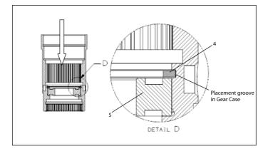
3. Grease Gear Case's (2) Splines with **Ingersoll Rand** # 90 Grease. Place spindle assembly (3) onto bearing in gear case with hand first and then press using manual press to butt against the placement face of bearing. Support bearing inner race during pressing. See section and detail views below for the proper placement.
