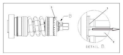
2. Insert The Bit of torx Driver (125116) in the teeth of Adjustment Nut and Nut Lock Washer's (17) Slot. Rotate torx Driver in Clockwise Direction to loose Adjustment Nut.
