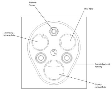
Note: The holes illustrated in above picture are for forward direction only. for reverse direction, secondary exhaust becomes the inlet and the inlet becomes the secondary exhaust.
