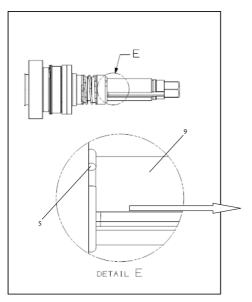
6. Remove Spring Guide (10), Collar Spring (2), Shut-off Collar (13) and Lower Jaw (14).
