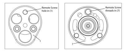
6. Insert Screw (9), Qty 2 in the counter holes in remote start housing of above assembly and tighten screws onto screw's threads in remote motor housing by hand first.
