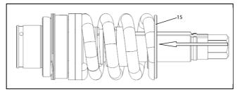
19. Grease both faces of Bearing (8) with Ingersoll Rand # 40036-1 grease and place over spring guide (15).
