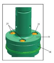
9. Grease ball groove of lower race (14) with Ingersoll Rand # 40036-1 Grease and slide on driver shaft (9).
