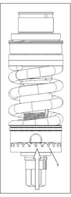
23. Insert the Bit of torx Driver (125116) in the teeth of adjustment nut and nut lock washer's (17) slot. Rotate torx driver in counter clockwise direction to tighten adjustment nut.
