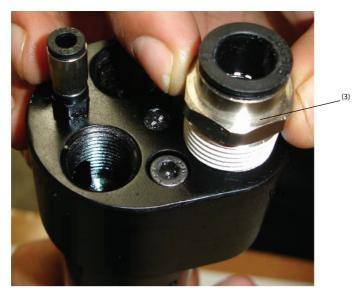
3. Tighten Tube Fitting (4) onto Inlet hole threads in Remote Backend Housing using spanner wrench.
