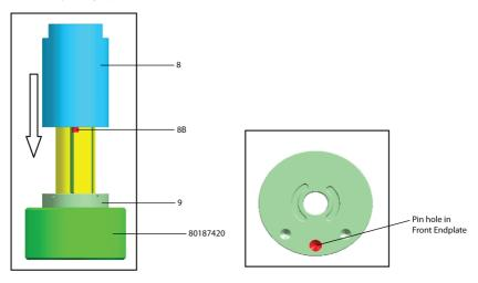
8. Put Rear Endplate Assembly onto rotor shaft. Align roll pin (7B) in rear endplate assembly with cylinder pin hole. **Note:** Counter Bore side of rear endplate assembly must be upward.
