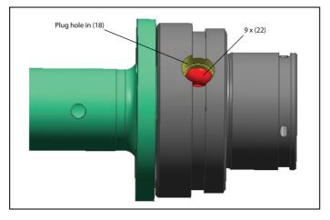
Place Plug (16) in plug hole of upper driven jaw (18). The smaller diameter of plug must face ball (22) inserted in step (3) Note: Plug must sit below the retaining ring surface of upper driven jaw.
