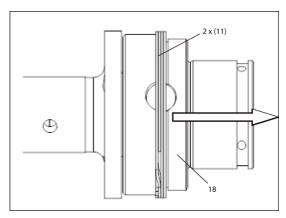
14. Remove Plug from driven jaw by tapping upper driven jaw gently against the work surface.
