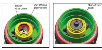
4. Grease O-ring (3) with Ingersoll Rand # 68 Grease. Mount It over The O-ring Groove (External) of Valve Seat (1) of above Assembly.
