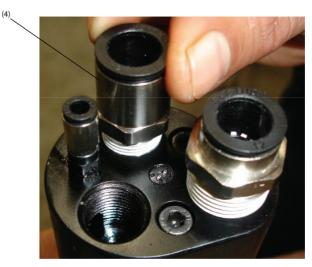
4. Tighten Tube fitting (4) onto Secondary exhaust hole threads in Remote Backend Housing using spanner wrench.
