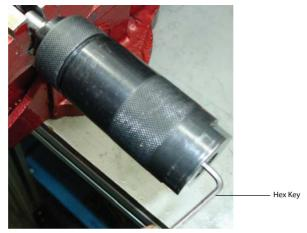
Remove Motor module from Motor Clamp Fixture 80187388 / 16604845.
