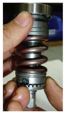
4. Remove Nut Lock Washer (17), Bearing (8), Spring Guide (15) and Clutch Spring (1).
