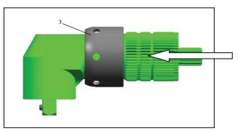
2. Place Coupling Nut Retainer (4) on the groove of angle housing of above assembly by using heavy duty retaining ring pliers.
