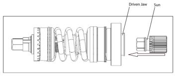
2. Insert Pin (QA6-15) into Upper Driven Jaw's pin hole to hold Sun in upper driven jaw. Pin must sit over the pin's groove in Sun.
