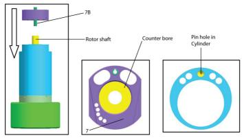
Grease Bearing (5) with Ingersoll Rand # 68 Grease and place onto Rotor Shaft and Rear Endplate Assembly counter Bore. Press Bearing Using Fixture 80187370 Until Assembly is tight and will not rotate.
