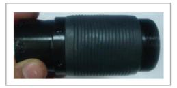
2. Orient Reverse Ring Assembly (7) with indicator hole closer to indicator hole on motor housing (1).
