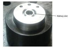
5. Place Rotor onto front endplate bore. Hold fixture 80187370 in manual press and press rotor in front endplate.
