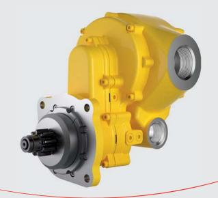
For engine displacement of: Diesel-0 to 600 CID (0 to 10 liters) Carbureted-0 to 1200 CID (0 to 20 liters)
