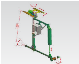
OSS = Overhead Rigid See-Saw Type
