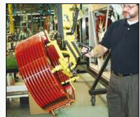
HVAC – copper coil
